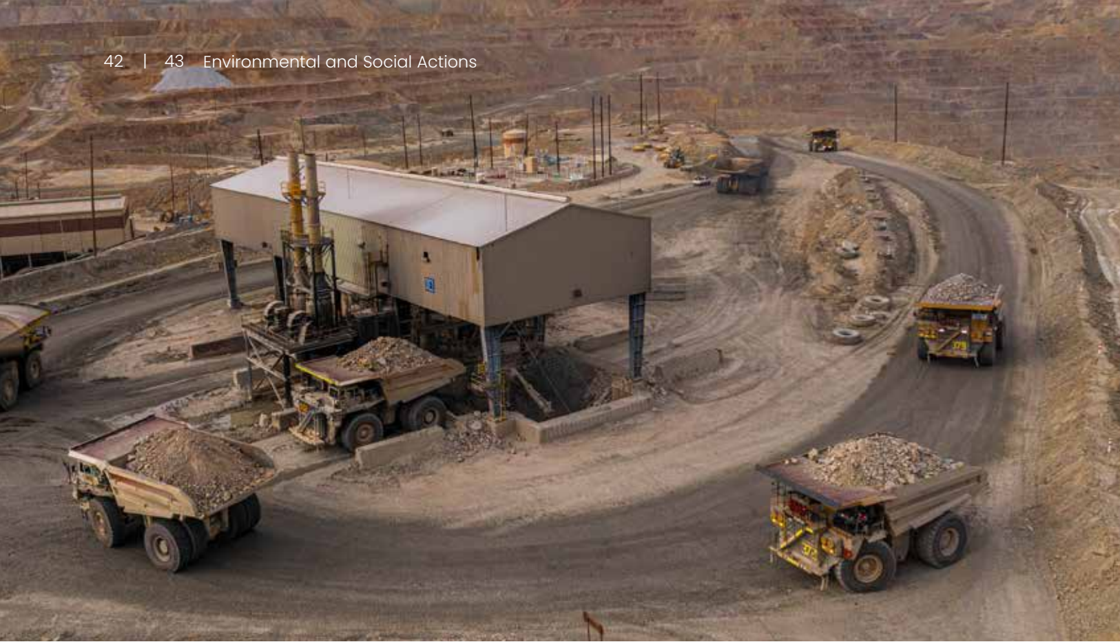
Energy-saving mining trucks with a capacity of up to 440 tons at the La Caridad mine in Nacozari de Garcia, Sonora, Mexico.
